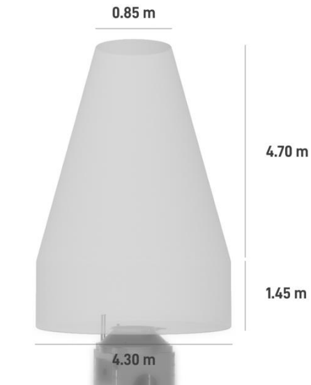
Figure 2-4: Cake Topper Payload Keep-In Volume (Clampband Configuration)
