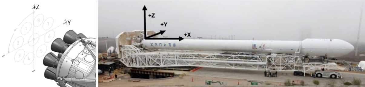
Figure 4-1: Launch Vehicle Coordinate Frame
