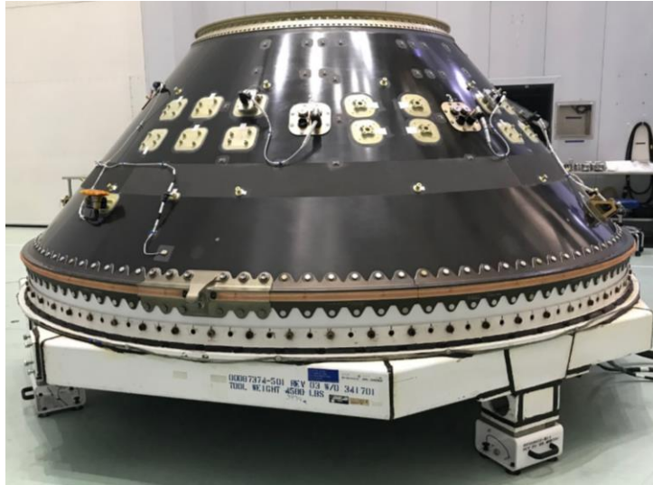
Figure 3-1: SpaceX 1,575-mm payload attach fitting
