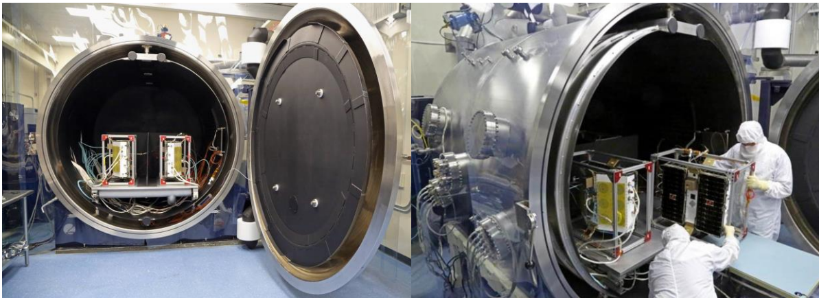
Figure 3. Thermal Vacuum Chamber. Credits: Southwest Research Institute - San Antonio, Texas.
