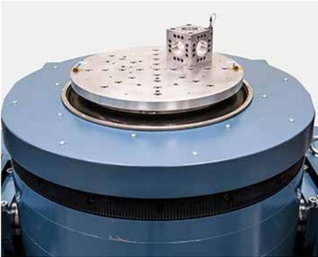
Experior Laboratories uses Unholtz-Dickie T-2000 vibration systems optimized for high G shaker shock up to 5,000G. Unholtz-Dickie vibration systems have inductively coupled solid metal coil armatures to prevent driver coil failure. Shakers with 3" stroke and 180 in/s of velocity allow for high G shock tests with large displacement requirements or short transients.
