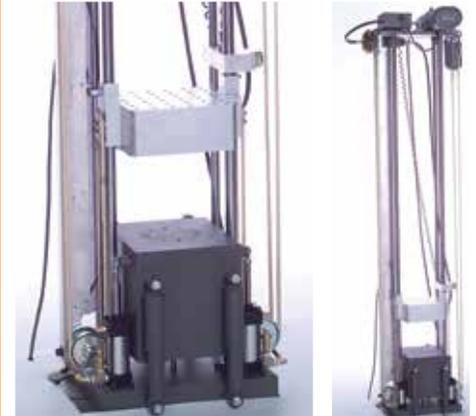
The Lansmont P30 shock system can produce half sine or haversine shocks in excess of 10,000G. Dual elastic accelerators boost the max velocity change to 600in/s or higher. The system comes with pneumatic brakes and a floating seismic base to allow durations as short as .15ms. Data is captured at 1MHz, with shock pulse amplitude and duration reported automatically. SRS plot generation is available.
