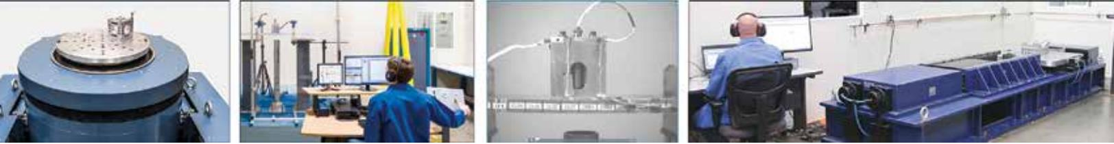
**Experior Laboratories'** MIL-STD-790 approved and ISO-17025:2005 accredited laboratory houses multiple state-of-the-art electrodynamic shaker and shock systems that can handle the most demanding test specifications.
