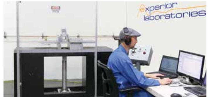
Experior Laboratories Kinetic Impact Pyroshock Simulation (KIPS) test system is able to simulate near and mid field Pyroshock, experienced by the parts closest to a pyrotechnic event, by using high speed impact to excite a tunable resonant beam. By adjusting the impact force, location, and damping, this platform allows for highly customizable shock generation. Our pneumatic system allows for quick setup and reset.
