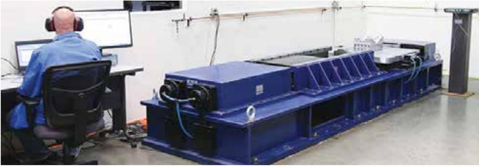
Experior Laboratories' horizontal shock system represents a dramatic increase in the size of units that can undergo SRS Shock testing. Parts mount to a 40"x40" platform that matches directly with slip tables on our high power T2000
