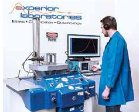
Classical Shock tests such as half-sine, sawtooth, and trapezoidal pulses are associated with product handling events (drop impacts) and transportation induced events (road bumps, pot holes, etc.) and are performed using our AVCO pneumatic shock table or any of our Unholtz-Dickie electrodynamic vibration systems. These shock tests are specified in the Time Domain (acceleration vs. time). Classical shock pulses up to 1,500G can be accommodated for a wide range of test payloads.
