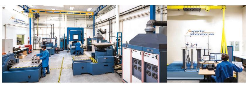
**Experior Laboratories**' MIL-STD-790 approved and ISO-17025:2005 accredited laboratory houses multiple state-of-the-art electrodynamic vibration shaker systems that can handle the most demanding vibration and shock test specifications.
