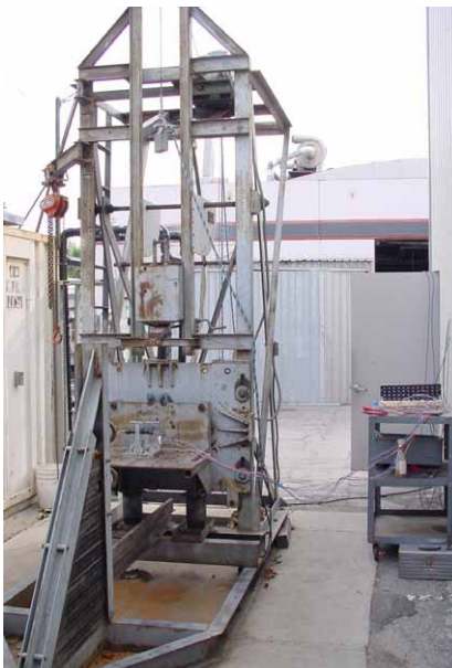
Figure 3: MIL-S-901 Hammer Shock test with fiber optic connector assembly
