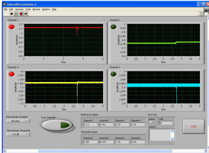
Figure 2: Measurements of signal discontinuities (as often required during military connector qualification testing)
